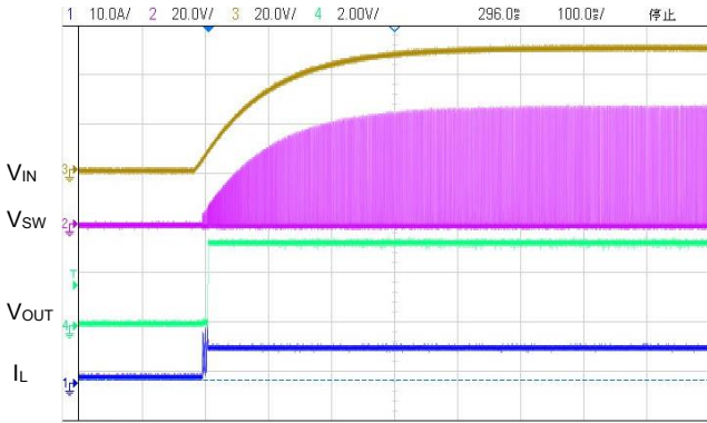
(19) Power Ramp Up (VIN=50.0V, VOUT=3.3V, IOUT=0.6A)
