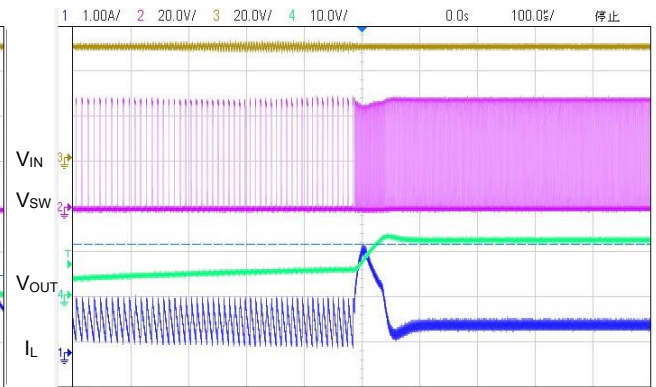
(22) Short Output Recovery (VIN=50.0V, VOUT=12V, IOUT=0.6A)
