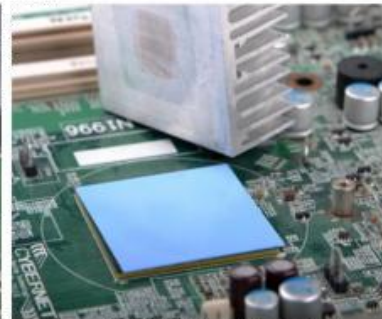
CP-120-T300 Series Thermal Thermal conductivity 3.0 W/m·K Double-sided adhesive Good electrical insulation Shockproof and vibration damping Good temperature resistance High cost-performance
