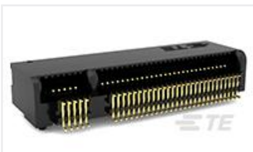
TE Part #1-2199230-6 M.2 0.5PITCH 4.2H KEY M 30U AU
