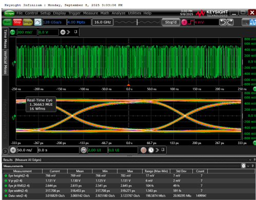
Figure 7. 3 Gbps Eye Diagram
