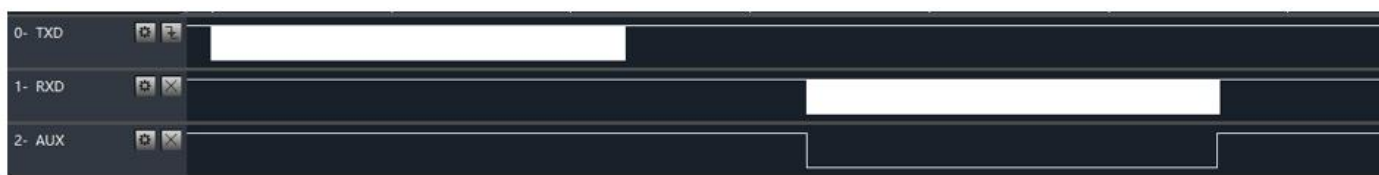
Timing sequence chart of AUX when RF receives data and send to MCU
