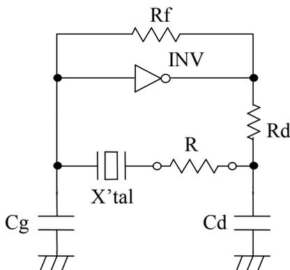
(1) Connect the resistor( $R$ ) to the circuit in series with the crystal unit.
