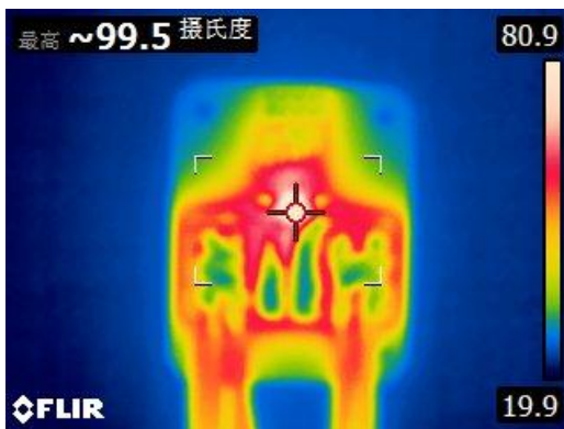
Package Thermography (Input Current 40A)
