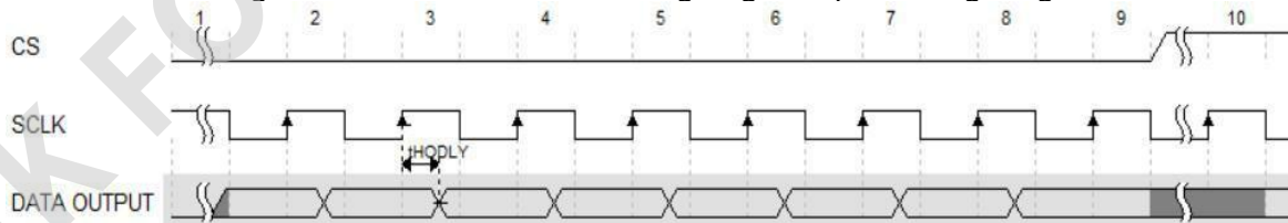
Figure 12-3. HSOD=1 Data Rising Edge Output Timing Diagram
