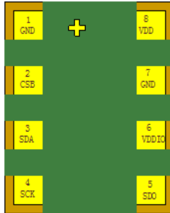
Figure 5: Layout pin configuration DPS368XTSA1 (Bottom View)
