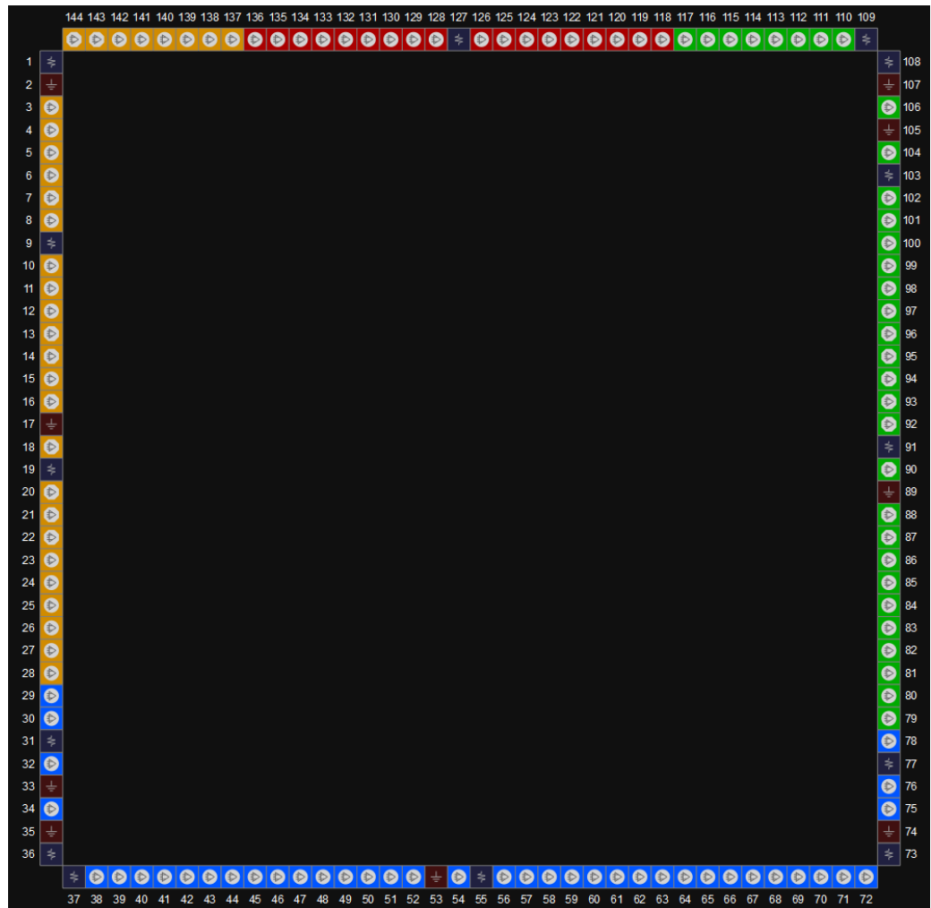
Figure 3-11 View of GW1NR-9 LQ144P Pins Distribution (Top View)
