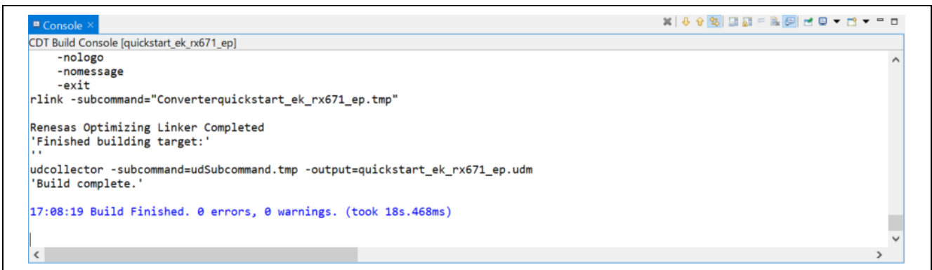
Figure 24. Console screen when the build is successful
