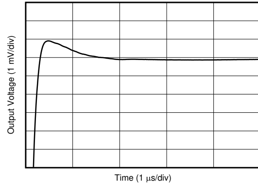
Figure 7-32. Large-Signal Settling Time (Positive)
