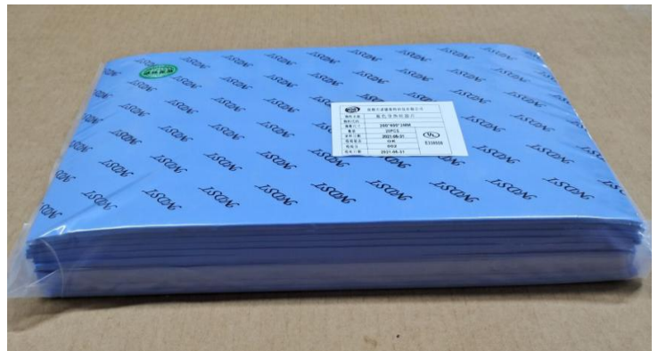
Place the product into a PE plastic bag and attach the inner packaging label
