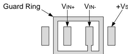
Figure 6. Example Guard Ring Layout for Inverting Comparator
