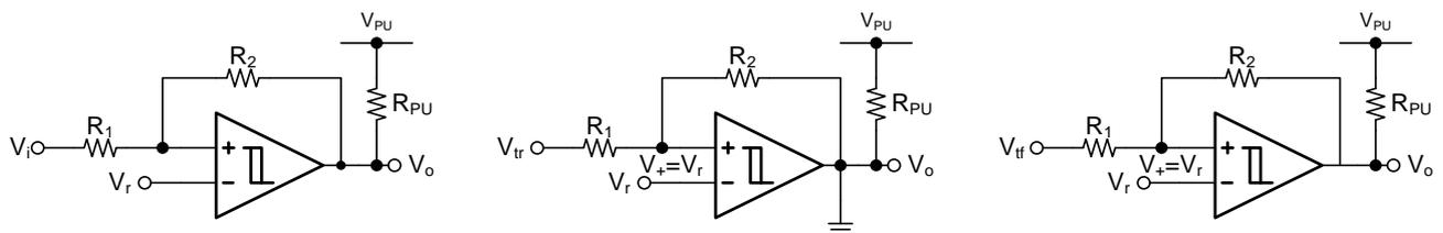
Figure 4. Non-Inverting Configuration with Hysteresis
