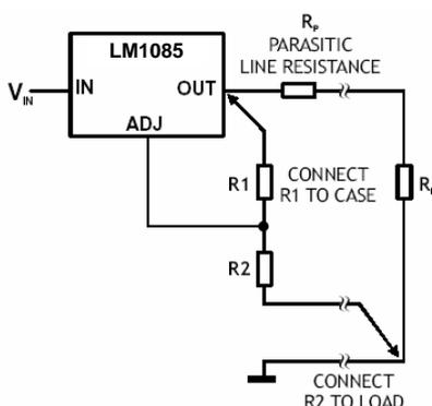
True remote load sensing it is not possible to provide, because the LM1085 is a three terminal device. The resistance of the wire connecting the regulator to the load will limit the load regulation.
