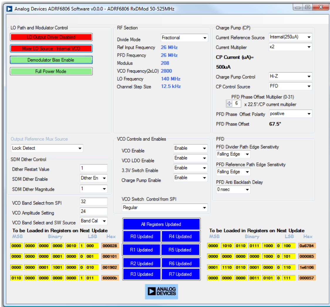
Figure 48. Evaluation Board Software Main Window
