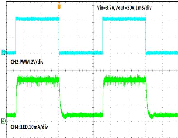
**PWM Dimming (20kHz)**
