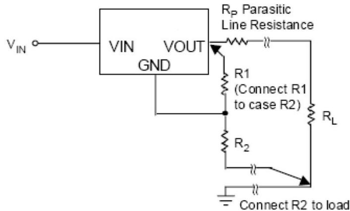
Figure 5. Best Load Regulation Using Adjustable Output Regulator
