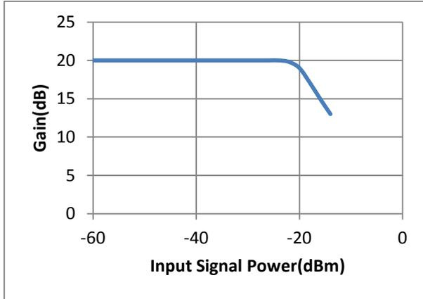
**Figure 7. Input P1dB Compression Point(P1dB)**
