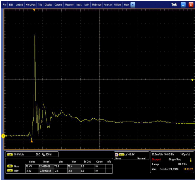
Figure 3. Positive 8kV contact per IEC 61000-4-2
