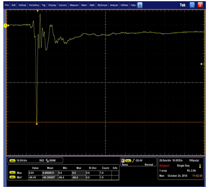
Fig 4. Negative 8kV contact per IEC 61000-4-2
