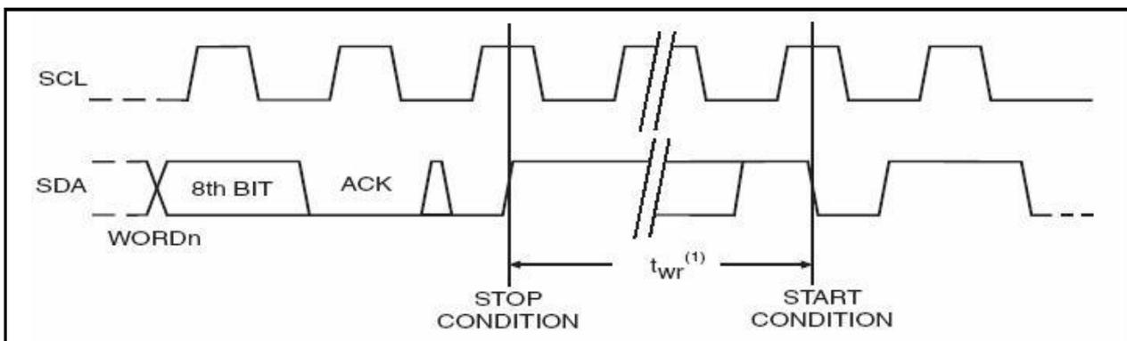
**Note:** 1. The write cycle time  $t_{WR}$  is the time from a valid stop condition of a write sequence to the end of the internal clear/write cycle.
